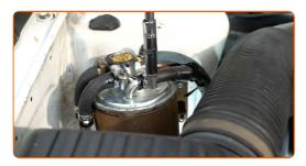
Disconnect the fuel supply lines from the fuel filter. Use round-nose pliers.
