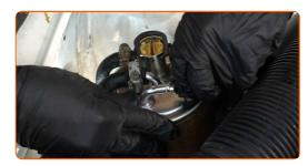
Screw the fastener attaching the fuel supply line to the fuel filter housing. Use a drive socket #7. Use a ratchet wrench.
