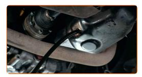
Replacement: engine oil and filter – VW Polo Hatchback (6R1, 6C1). AUTODOC recommends:
