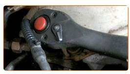
Remove the oxygen sensor.
