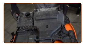
Screw in the fastening screws of the air filter cover. Use a Phillips screwdriver.
