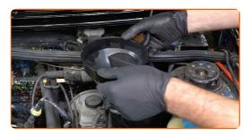
Pour coolant in the coolant reservoir.
