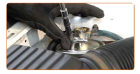
Fill the new filter with fuel. Use a hand-operated fluid syringe.
