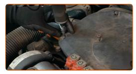
Remove the air filter housing.
