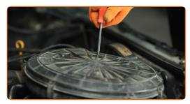
Release the air filter cover clips.
