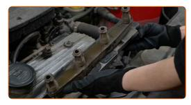
Clean dirt, dust and debris from inside the spark plug wells.
