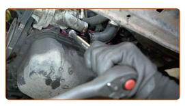
Remove the thermostat housing.
