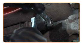
9 Remove the brake caliper. Use a crowbar.
