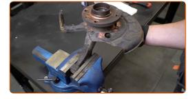
Clean the fasteners of the brake disc cover. Use a wire brush. Use WD-40 spray.
