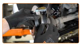
Clean the brake disc fasteners. Use a wire brush. Use WD-40 spray.
