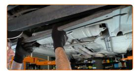
Screw in the fasteners of the plastic car body protective cover. Use a drive socket #10. Use a ratchet wrench.
