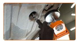
Remove the plastic car body protective cover.
