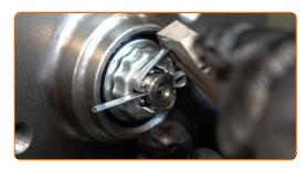
Install the cap of the hub nut. Use a rubber mallet.
