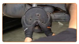
Clean the hub bearing mounting seat. Clean the hub. Use all-purpose cleaning spray.
