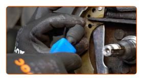
Compress the wheel cylinder. Use water pump pliers.
