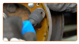
Install the lower return spring. Use a crowbar. Use a flat screwdriver.
