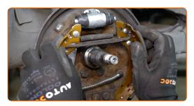
Reinstall the brake shoe hold-down cup. Use a brake shoe retaining spring compressor.
