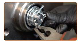
16 Install the cap of the hub nut. Use a rubber mallet.
