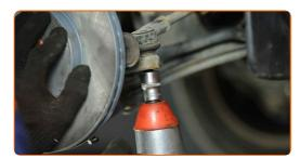
Treat the fastener connecting the tie rod end to the steering knuckle. Treat the fasteners of the ball joint. Use copper grease.
