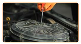
Release the air filter cover clips.
