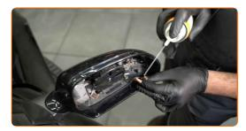
6 Attach the mirror heating connectors.
