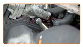
Remove the thermostat housing.
