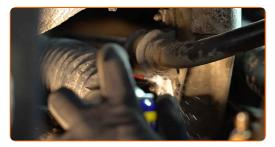
Unscrew the fasteners of the stabilizer bush brackets. Use a combination spanner #13.
