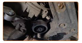
Screw in the engine mount fastener that connects it to the subframe. Use a drive socket #16.
