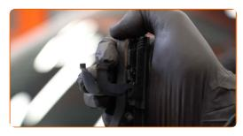
Remove the blade from the wiper arm.
