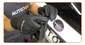
Remove the blade from the wiper arm.
