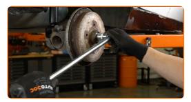
Remove the brake drum assembled with the wheel hub bearing. Use a flat screwdriver.
