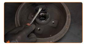
Remove the hub bearing mounting. Use a crowbar.
