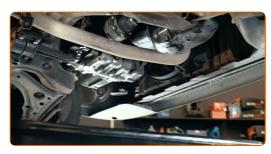
Clean the area of the oil pan drainage hole. Use a wire brush. Use all-purpose cleaning spray.
