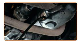
Replacement: engine oil and filter – VW POLO (6N2). AUTODOC recommends:
