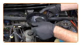
Pour coolant in the coolant reservoir.
