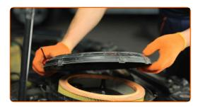
6 Remove the filter element from the filter housing.
