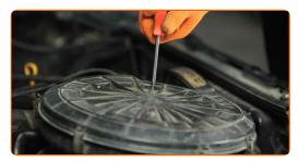
Release the air filter cover clips.
