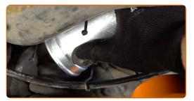
Attach the fuel filter fasteners. Use nippers.
