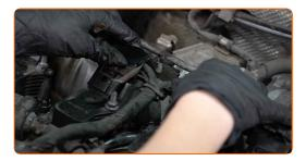
Connect the ground wires to the ignition coils and screw in the fasteners. Use a drive socket #10. Use a ratchet wrench.
