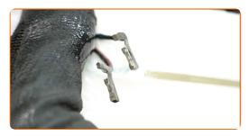
6 Attach the mirror heating connectors.
