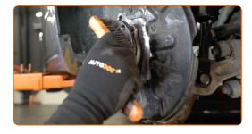
75 Install the brake disc.
