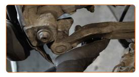
Screw the fasteners of the ball joint. Use a combination spanner #18.
