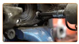
Remove the wheel hub from the steering knuckle.
