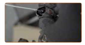
Connect the brake pad wear sensor plug.
