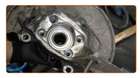
Tighten the hub. Use XZN #12. Use a torque wrench. Tighten it to 80 Nm torque.+90°
