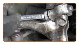
28 Remove the fastening bolt.
