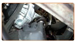
Replacement: engine thermostat – VW PASSAT Variant (3B5). Tip:
