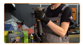
Screw the shock strut piston rod upper fastening. Use a combination spanner #17. Use locking pliers. Use a torque wrench. Tighten it to 25 Nm torque.
