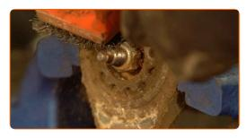
Remove the shock absorber piston rod fastening. Use a shock absorber socket #5. Use a drive socket #17. Use a ratchet wrench.
