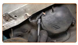
Remove the oxygen sensor housing cover.
