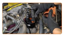
Replacement: distributor cap – VW PASSAT Variant (3B5). Tip:
