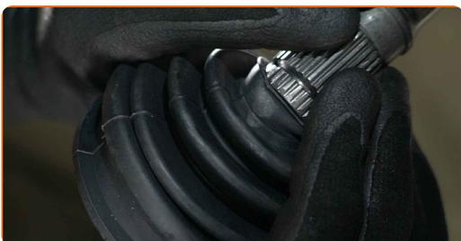
**33** Install the CV joint circlip.
