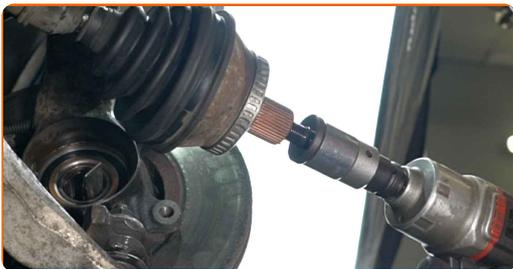
**26** Unscrew the fastener connecting the drive shaft to the wheel hub.
