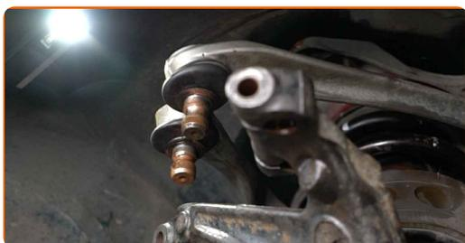
**20** Disconnect the tie rod end from the steering knuckle.
