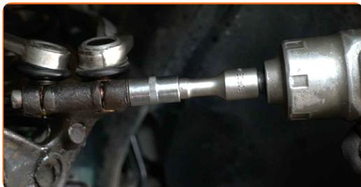
**50** Tighten the upper arm fastenings. Use a drive socket #16. Use HEX No.H8. Use a torque wrench. Tighten it to 40 Nm torque.
