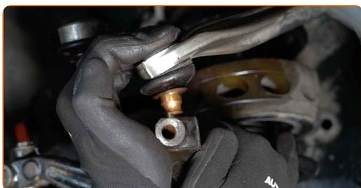
**48** Install the fastening bolt. Use a crowbar.
