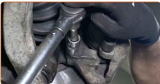
**56** Treat all joints of the arm. Treat the steering knuckle fasteners. Use copper grease.
