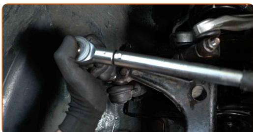
**52** Install and tighten the drive shaft bolt. Use a drive socket #27. Use a ratchet wrench.
