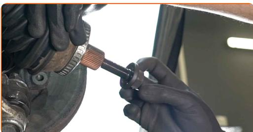
**28** Remove the CV joint together with its boot.
