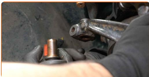
**21** Remove the fastening bolt. Use a drive socket #27.
