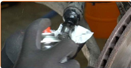
**31** Remove the CV joint circlip. Use a flat screwdriver.
