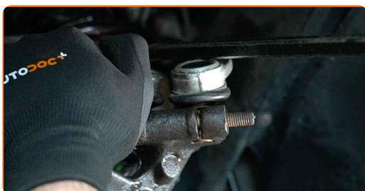
**49** Screw in the fasteners of the upper control arms. Use a drive socket #16. Use HEX No.H8. Use a ratchet wrench.
