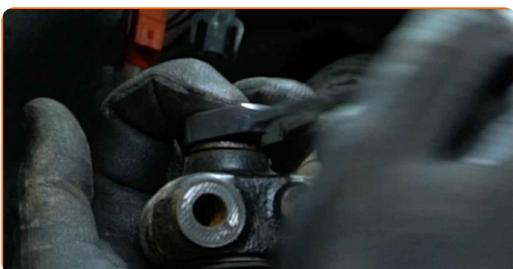
**15** Remove the fastening bolt. Use a pin punch. Use a hammer.
