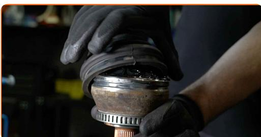
**30** Clean the CV joint mounting seat. Use all-purpose cleaning spray.
