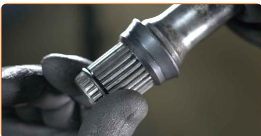
**34** Pack the CV joint with the grease supplied in the kit.
