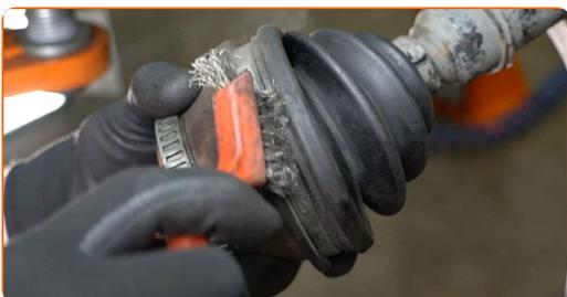
**24** Detach the clamps of the CV joint boot. Use a flat screwdriver.
