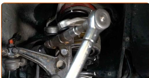
**51** Tighten the tie rod end fastening bolt. Use a drive socket #16. Use a torque wrench. Tighten it to 45 nm torque.
