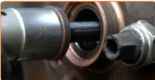
**22** Detach the driveshaft from the steering knuckle.
