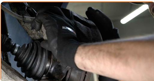
**55** Tighten the brake caliper bracket. Use a drive socket #17. Use a torque wrench. Tighten it to 130 Nm torque.
