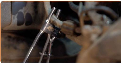
**9** Put a container for gathering brake fluid beneath.
