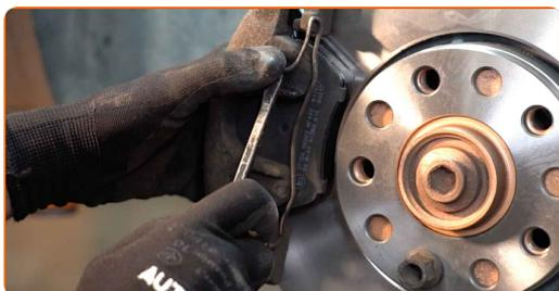
**15** Remove the brake caliper.
