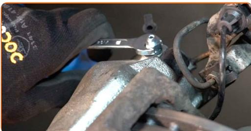
**33** Connect the brake bleeder kit to the brake bleeder screw.
