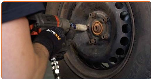
**42** Lower the car and working in a cross order, tighten the wheel bolts. Use a torque wrench. Tighten it to 120 Nm torque.
