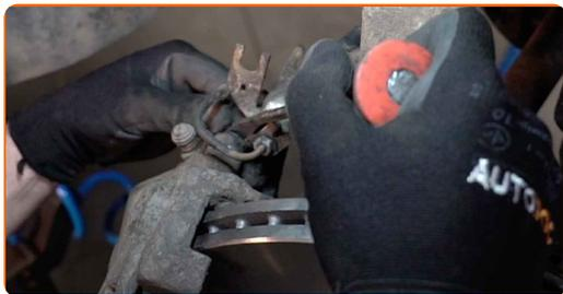
**13** Unscrew the brake caliper fastening. Use HEX No.H7. Use a ratchet wrench.
