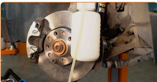
32 Undo the brake bleeder screw. Use a combination spanner #10.
