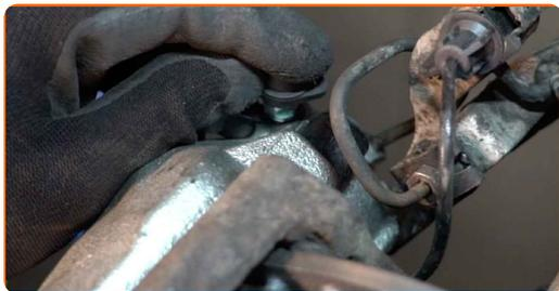
**34** Bleed the brake caliper system. Without starting the engine, press the brake pedal several times until you feel significant resistance.
