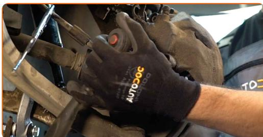
**14** Detach the brake caliper retaining spring. Use a crowbar.
