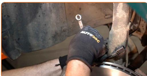
28 Remove the brake hose clamp.
