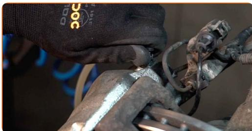
**37** Tighten the brake caliper bleed screw. Use a drive socket #10. Use a torque wrench. Tighten it to 9 Nm torque.
