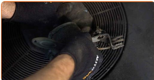
**19** Unscrew the fastener connecting the brake pipe to the brake caliper. Use a combination spanner #11.
