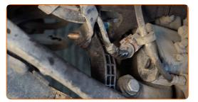
13 Screw the fasteners of the stabilizer bush brackets. Use a combination spanner #15. Use a drive socket #15. Use a torque wrench. Tighten it to 35 Nm torque.
