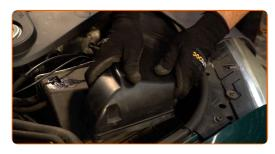
Release the air filter cover clips.
