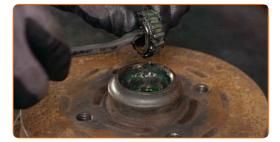
Remove the inner oil seal of the wheel bearing. Use a crowbar.
