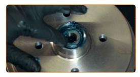
Treat the wheel hub in the area where it contacts the brake drum. Use a multipurpose grease.
