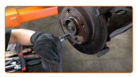
Remove the brake disc.
