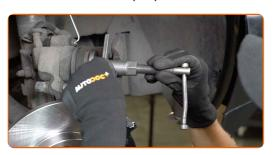
Install the brake caliper and fix it. Use HEX No.H6. Use a torque wrench. Tighten it to 25 Nm torque.
