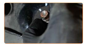
Screw in the fastener connecting the control arm to the subframe. Use a drive socket #18. Use a ratchet wrench.
