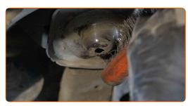
Install the rubber spacer on the new coil spring.
