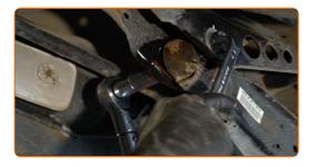
Remove the support from under the arm.
