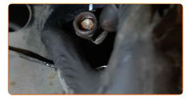
Remove the support from under the arm.
