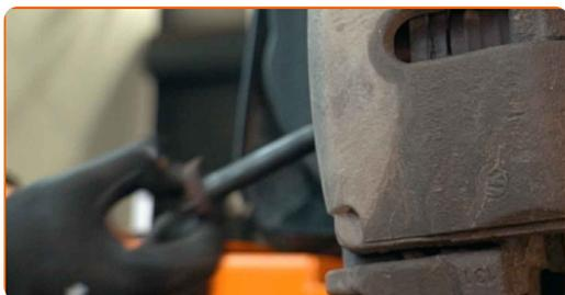
**20** Unscrew the lower fastener connecting the shock strut to the steering knuckle. Use a drive socket #18. Use XZN #14. Use a ratchet wrench.
