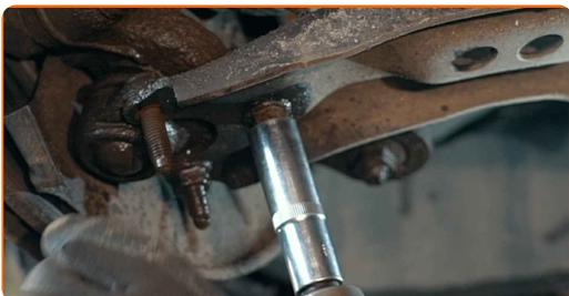
**23** Disconnect the ball joint from the arm. Use a crowbar.
