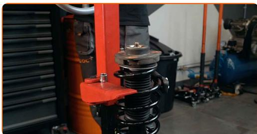
48 Remove the assembled shock strut.
