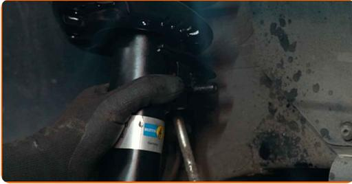
**66** Tighten the fastener connecting the stabilizer link to the shock strut. Use a combination spanner #18. Use a drive socket #18. Use XZN #6. Use a torque wrench. Tighten it to 55 Nm torque.
