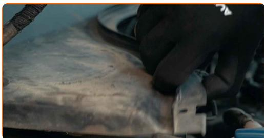
6 Clean the fasteners of the shock strut upper mount. Use a wire brush. Use WD-40 spray.
