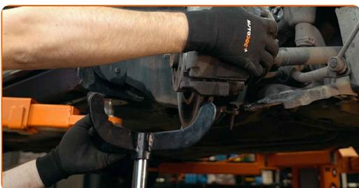
**25** Detach the driveshaft from the steering knuckle. Use a pin punch. Use a hammer.
