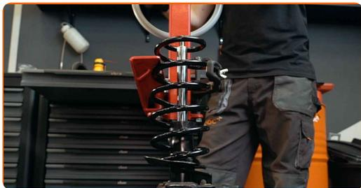
**43** Install the dust sleeve and the bump stop on the new shock absorber.
