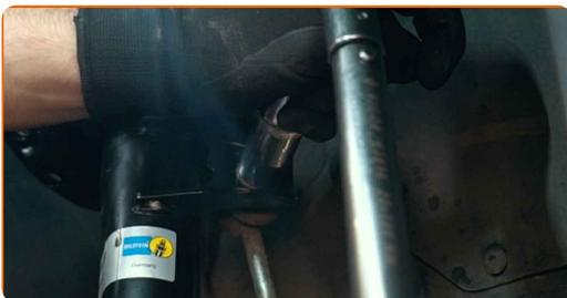
**67** Install and tighten the drive shaft bolt. Use a drive socket #27. Use a ratchet wrench.
