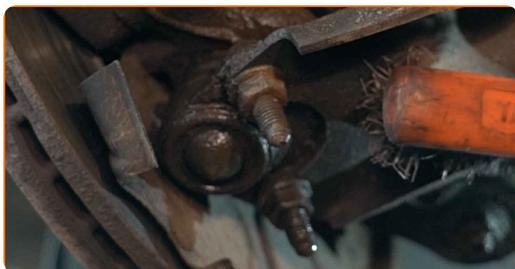
**22** Unscrew the fastener connecting the ball joint to the suspension control arm. Use a drive socket #16. Use a ratchet wrench.
