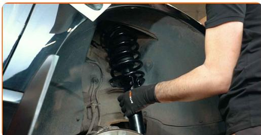
**51** Secure the upper fasteners of the shock strut. Do not tighten it.
