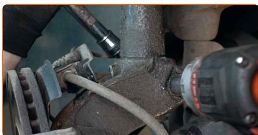
**21** Clean the fasteners connecting the ball joint to the suspension control arm. Use a wire brush. Use WD-40 spray.
