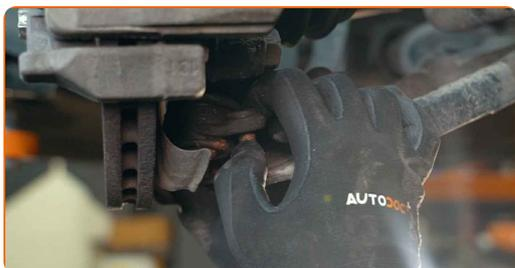
**61** Tighten the fasteners connecting the ball joint to the control arm. Use a drive socket #16. Use a torque wrench. Tighten it to 60 Nm torque.
