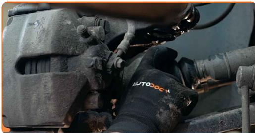
**59** Clean the ball joint mounting seat. Use a wire brush. Use WD-40 spray.
