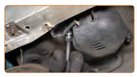
Remove the oxygen sensor housing cover.
