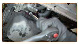
Remove the thermostat housing.
