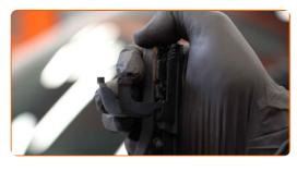
Remove the blade from the wiper arm.
