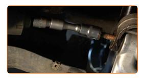
Install the rear fastener of the control arm (2 pieces).
