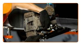
11.1 Unscrew the brake caliper fastening.
