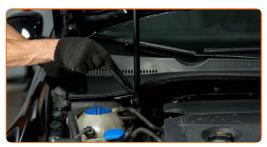
Clean the fasteners of the shock strut upper mount. Use WD-40 spray.
