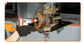
Install the transverse stabilizer link. Tighten the fastener connecting the stabilizer link to the shock strut. Use a drive socket #19. Use a torque wrench. Tighten it to 60 Nm torque.
