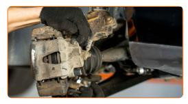
Connect the wiring and the brake hose to the bracket on the steering knuckle.
