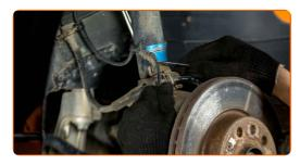
Remove the dust boot caps of the brake caliper guide pins. Use a flat screwdriver.
