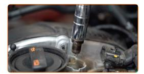
Apply a thin layer of a special high temperature anti-seize lubricant to the threads of the new spark plugs. Treat the surface of the terminals of the new spark plugs. Use high-temperature grease.
