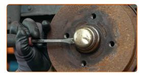
Remove the cotter pin securing the hub nut. Use a crowbar. Use a hammer.
