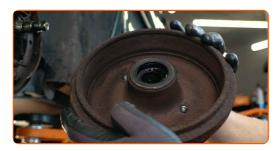
Clean the hub bearing mounting seat. Use all-purpose cleaning spray.
